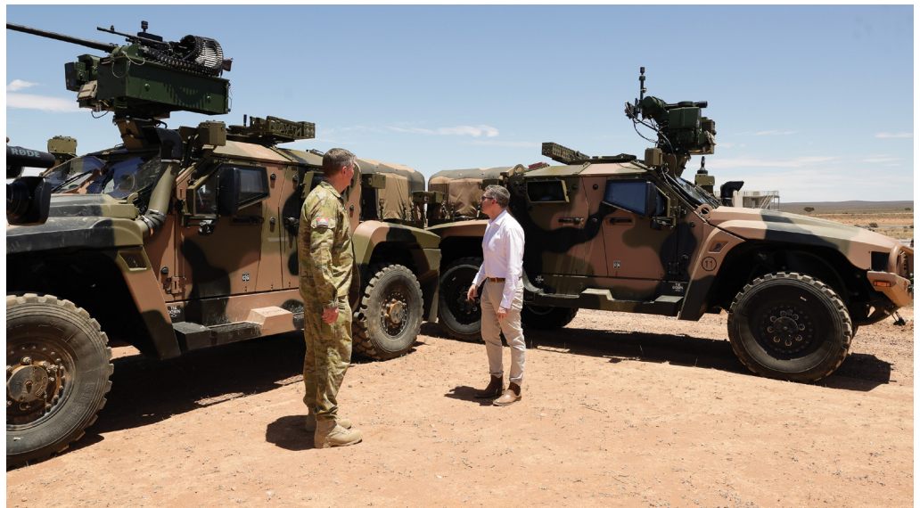
EOS Slinger remote weapon stations are here mounted on Hawkei vehicles – one armed with a 7.62mm machine gun/M230LF 30mm cannon combination, and the other an M134D Minigun – at Land 156's Capability Target State 1 demonstration in December 2025. (ADF)
