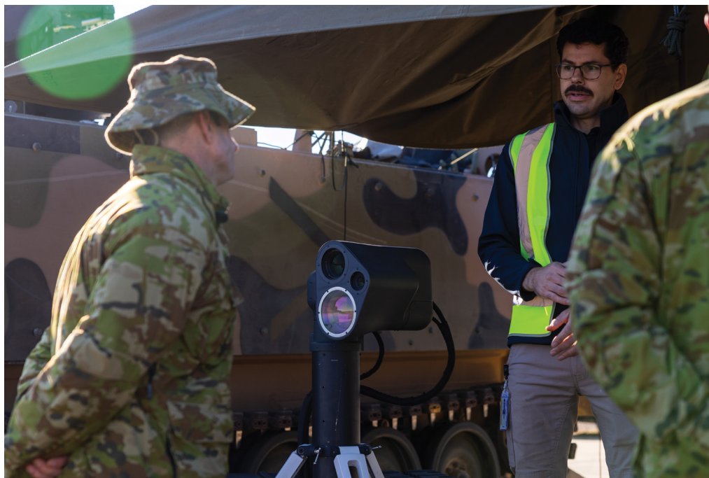
The Portable Fractl Laser Weapon System from AIM Defence underwent its first successful testing in May 2024. Directed-energy weapons offer some advantages when integrated into wider C-UAS systems. (ADF)
