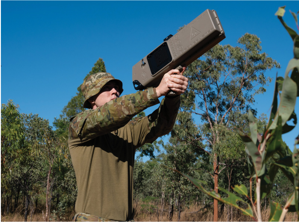
Soldiers deployed in Joint Task Force 629 in Weipa recently tested and trained with counter-drone technology during Exercise Austral Shield 2026. This is a DZYNE Dronebuster DB-4 jammer. (ADF)
