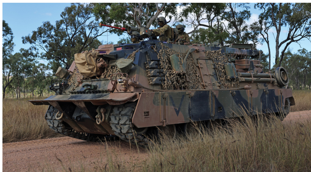
All the new heavy armour arriving in the Australian Army requires bolstered support, such as M88A2 HERCULES recovery vehicles. (Gordon Arthur)
